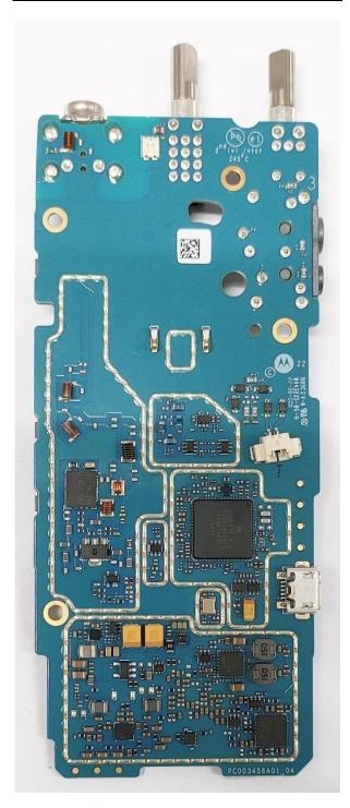
Exhibits 9C - RF board with Shields (Bottom)
