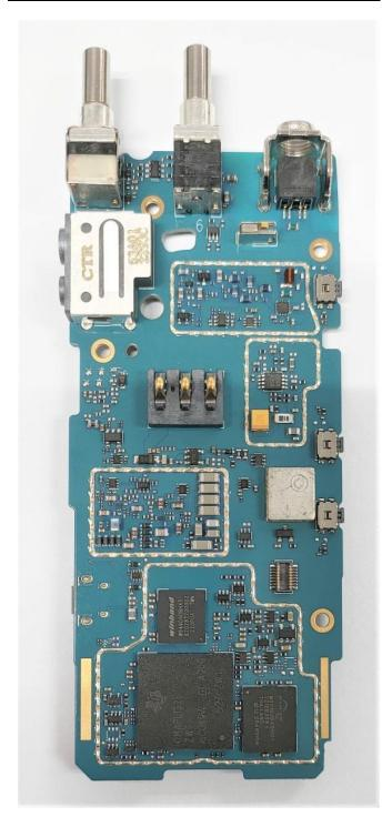
Exhibit 9E - RF board with chassis and housing (Front side)
