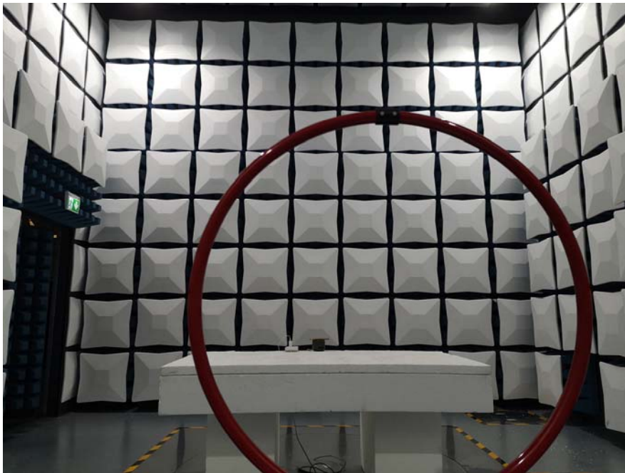
Radiated Emissions (Above 30MHz)
