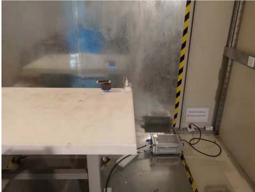
Conducted Emissions (Side View)
