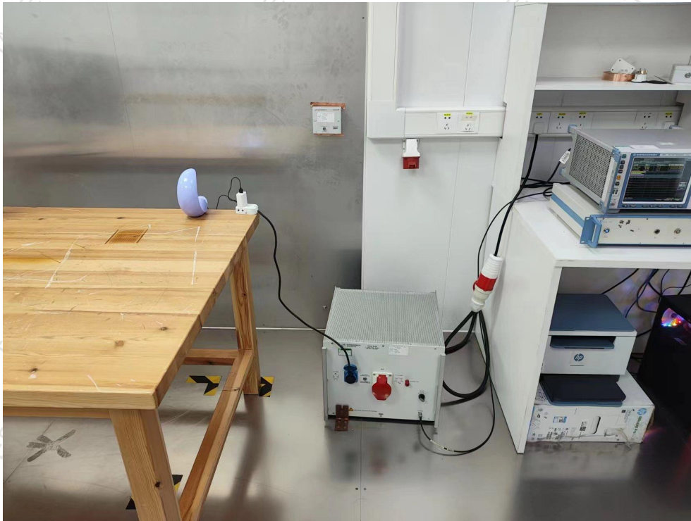
Photo of Conducted Emission Measurement
