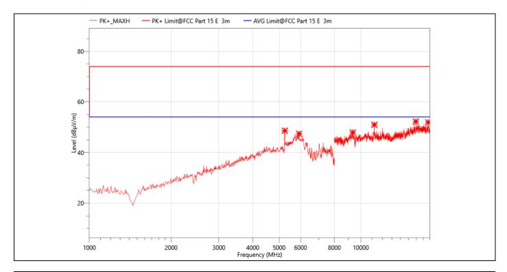
**EUT: Smart Projector** Temperature: **24.3℃** M/N.: HY300 **Humidity:** 54%RH **Power Rating:** Mode: 802.11a 5825MHz AC 120V/60Hz **Test Engineer: Test Time:** 2023-08-30 **Berny**
