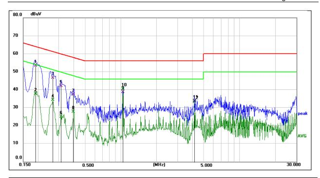
Phase: **EUT: Smart Projector** N M/N.: HY300 **Temperature:** 26°C Mode: 802.11ax HE20 5240MHz **Humidity:** 54%RH **Test Engineer:** Aiden **Power Rating:** AC120V/60Hz
