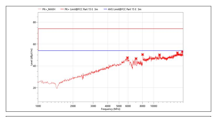
**EUT: Smart Projector** Temperature: **24.3℃** M/N.: HY300 **Humidity:** 54%RH **Power Rating:** Mode: 802.11ax HE20 5180MHz AC 120V/60Hz **Test Engineer: Test Time:** 2023-08-30 **Berny**
