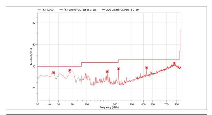
EUT: Smart Projector Temperature: 24.3℃ M/N.: HY300 **Humidity:** 54%RH Mode: 802.11ax HE20 5240MHz **Power Rating:** AC 120V/60Hz Berny **Test Time: Test Engineer:** 2023-08-30
