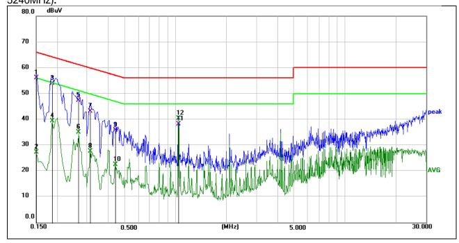
EUT: **Smart Projector** Phase: L1 M/N.: **HY300 Temperature:** 26℃ Mode: 802.11ax HE20 5240MHz **Humidity:** 54%RH **Test Engineer:** Aiden **Power Rating:** AC120V/60Hz
