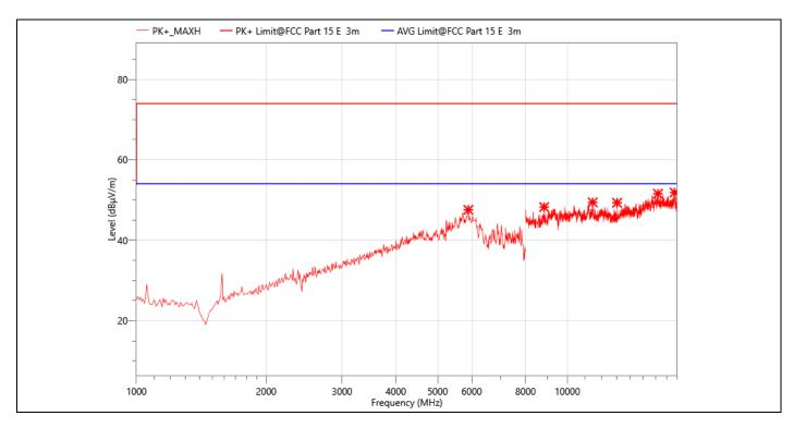
**EUT: Smart Projector Temperature:** 24.3℃ M/N.: HY300 **Humidity:** 54%RH 802.11a 5825MHz **Power Rating:** Mode: AC 120V/60Hz **Test Time: Test Engineer: Berny** 2023-08-30
