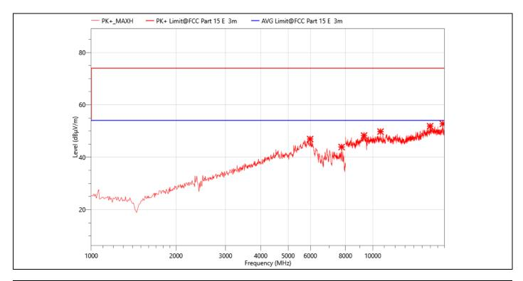
Temperature: **EUT: Smart Projector 24.3℃** M/N.: HY300 **Humidity:** 54%RH **Power Rating:** Mode: 802.11a 5785MHz AC 120V/60Hz **Test Engineer: Test Time:** 2023-08-30 **Berny**
