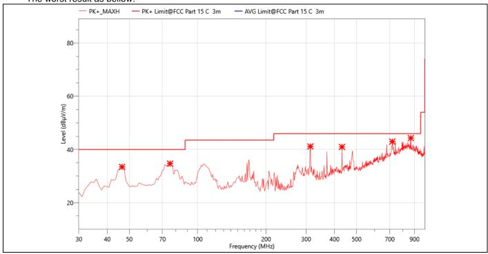
**EUT:** Temperature: **Smart Projector** 24.3℃ M/N.: HY300 **Humidity:** 54%RH Mode: 802.11ax HE20 5240MHz **Power Rating:** AC 120V/60Hz **Test Time: Test Engineer:** 2023-08-30 **Berny**
