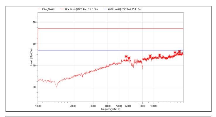
**EUT: Smart Projector Temperature:** 24.3℃ M/N.: HY300 **Humidity:** 54%RH 802.11ax HE20 5240MHz **Power Rating:** Mode: AC 120V/60Hz **Test Time: Test Engineer: Berny** 2023-08-30
