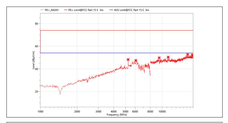
**EUT: Smart Projector** Temperature: **24.3℃** M/N.: HY300 **Humidity:** 54%RH **Power Rating:** Mode: 802.11ax HE20 5240MHz AC 120V/60Hz **Test Engineer: Test Time:** 2023-08-30 **Berny**
