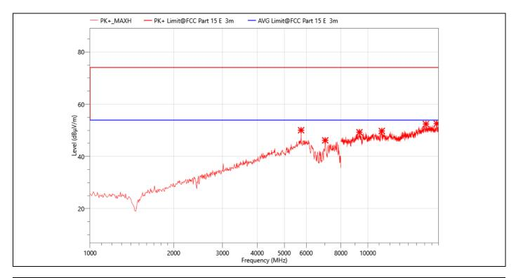
**EUT: Smart Projector** Temperature: **24.3℃** M/N.: HY300 **Humidity:** 54%RH **Power Rating:** Mode: 802.11ax HE20 5200MHz AC 120V/60Hz **Test Engineer: Test Time:** 2023-08-30 **Berny**
