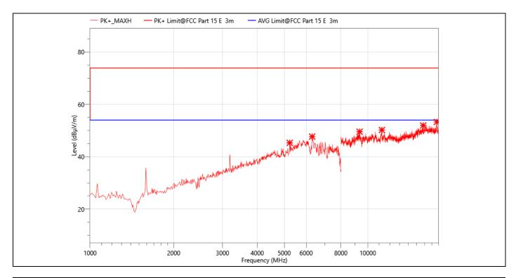
**EUT: Smart Projector** Temperature: **24.3℃** M/N.: HY300 **Humidity:** 54%RH Mode: 802.11a 5745MHz **Power Rating:** AC 120V/60Hz **Test Engineer: Test Time:** 2023-08-30 **Berny**
