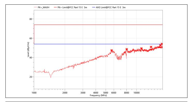
**EUT: Smart Projector Temperature:** 24.3℃ **Humidity:** M/N.: HY300 54%RH **Power Rating:** Mode: 802.11ax HE20 5180MHz AC 120V/60Hz **Test Engineer: Berny Test Time:** 2023-08-30
