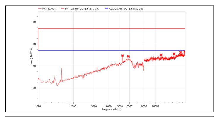
EUT: **Smart Projector** Temperature: 24.3℃ M/N.: HY300 **Humidity:** 54%RH **Power Rating:** Mode: 802.11a 5745MHz AC 120V/60Hz **Test Engineer: Test Time:** Berny 2023-08-30
