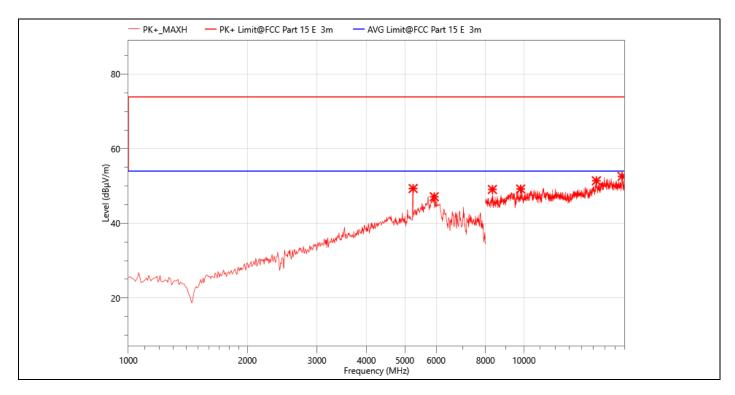
**EUT: Smart Projector** Temperature: **24.3℃** M/N.: HY300 **Humidity:** 54%RH **Power Rating:** Mode: 802.11a 5785MHz AC 120V/60Hz **Test Engineer: Test Time:** 2023-08-30 **Berny**
