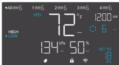
Either of the two trigger points can activate while you are in VPD Mode, even if you are viewing another trigger point. Set a trigger point to OFF if not in use, by holding down the up and down buttons.
