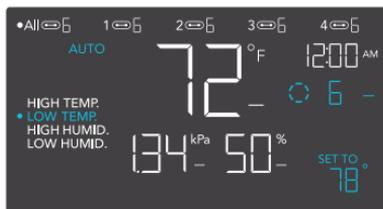
Any of the four trigger points can activate while you are in AUTO Mode, even if you are viewing another trigger point. Set a trigger point to OFF if not in use, by holding down the up and down button.
