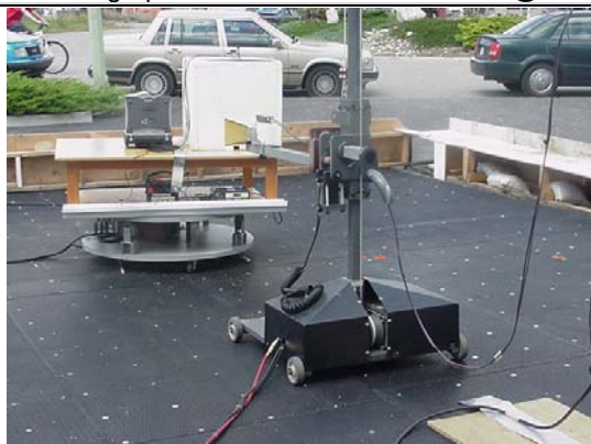
Photograph F-11 - 3115 Horn with LNA @ 1m
