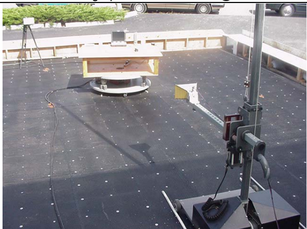
Photograph F-5 - 3115 Horn with LNA @ 1m
