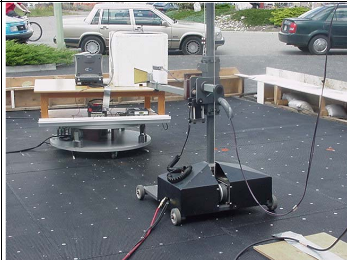
Photograph E-6 - Standard Gain Horn @ 1 m
