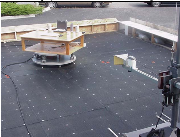
Photograph F-6 - Standard Gain Horn @ 1m
