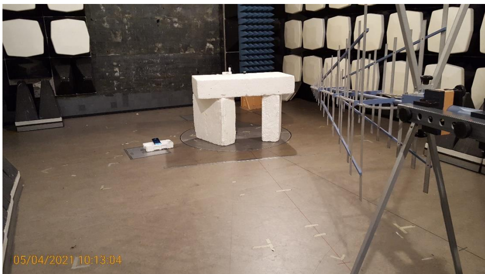
Photo 3. Radiated emission test setup. 30 – 1000 MHz.
