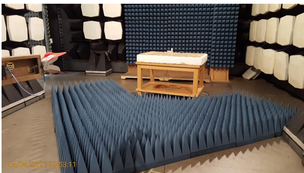
Photo 4. Radiated emission test setup. 1 - 18 GHz.
