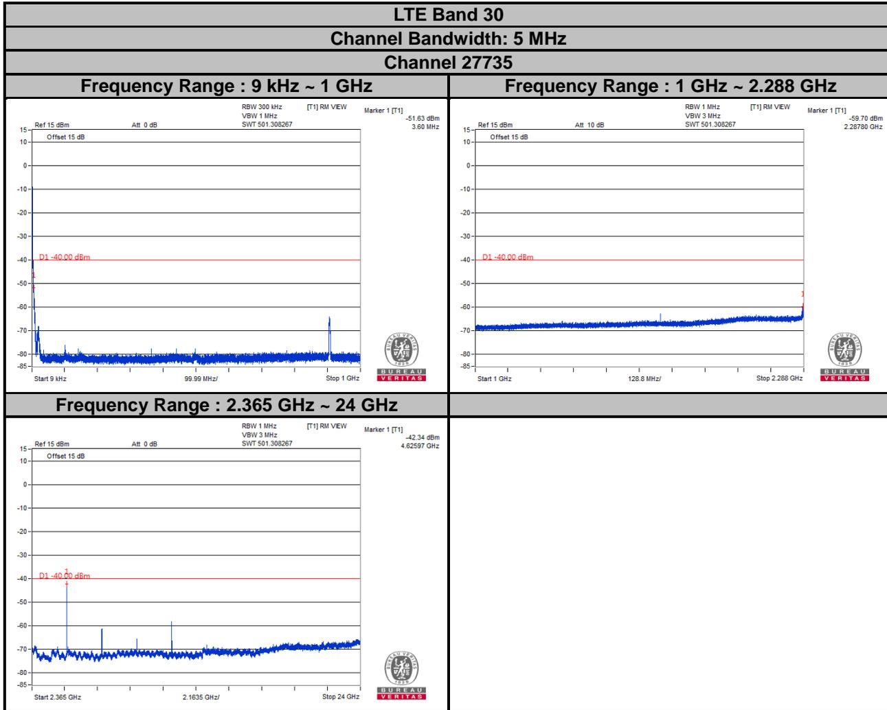
Note: The signal over the limit in 9 kHz is from spectrum analyzer.
