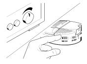
ADJUSTING THE RECEIVER CHANNEL Turn the TUNE control on the earpiece until you can hear the audio signal loud and clear.
