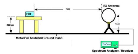
For radiated emissions from 30MHz to 1GHz
