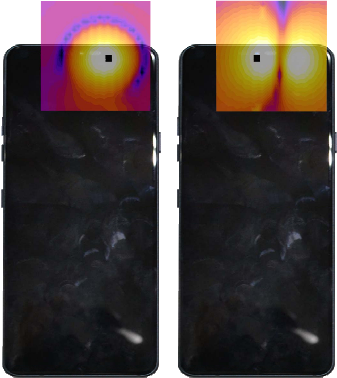
Figure 16-3 T-Coil Scan Overlay Magnetic Field Distributions
