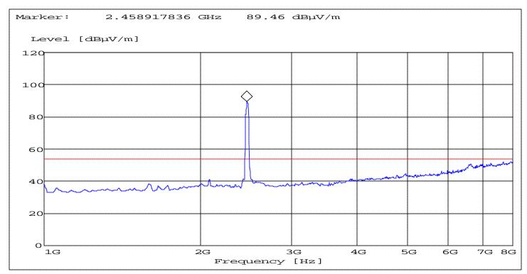
NOTE: The marked peak is the carrier frequency. Frequency resolution is not fine enough to show the exact frequency of the carrier, refer to plots under EIRP.
