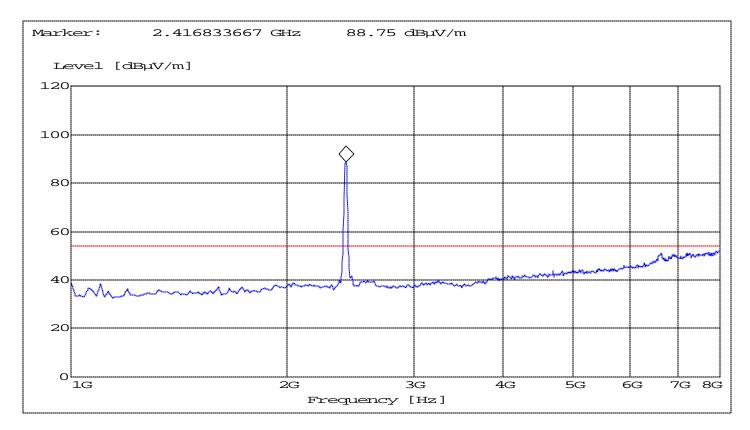
NOTE: The marked peak is the carrier frequency. Frequency resolution is not fine enough to show the exact frequency of the carrier, refer to plots under EIRP.
