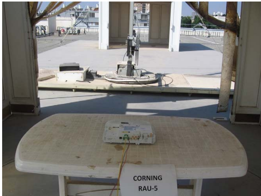
Figure 5. Radiated Emission Test
