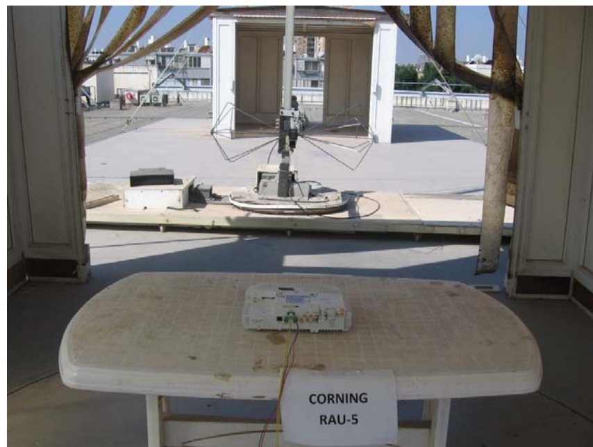
Figure 4. Radiated Emission Test
