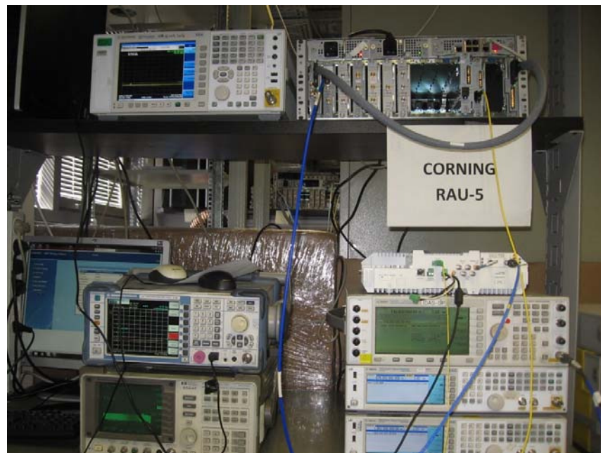
Figure 3. Conducted Emission From Antenna Port Tests
