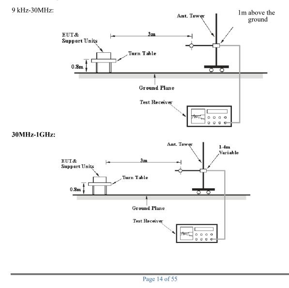
The radiated emission tests were performed in the 3-meter chamber test site, using the setup accordance with the ANSI C63.10-2013.
