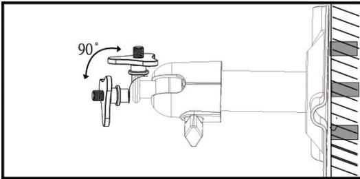
Loosen up the Thumb screw. Adjust proper view angle then secure the joint with T-bolt.
