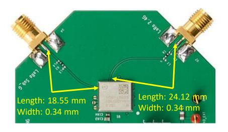
PCB for assembly the antenna
