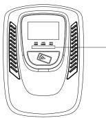
Waiting for Charging - Green Light After the vehicle connector is connected to the vehicle inlet, the CHARGE light is constantly lit.
