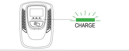
Step 5 / Charging Finished When the charging is finished, the green light (CHARGE) is constantly lit, please press the button on connector.
