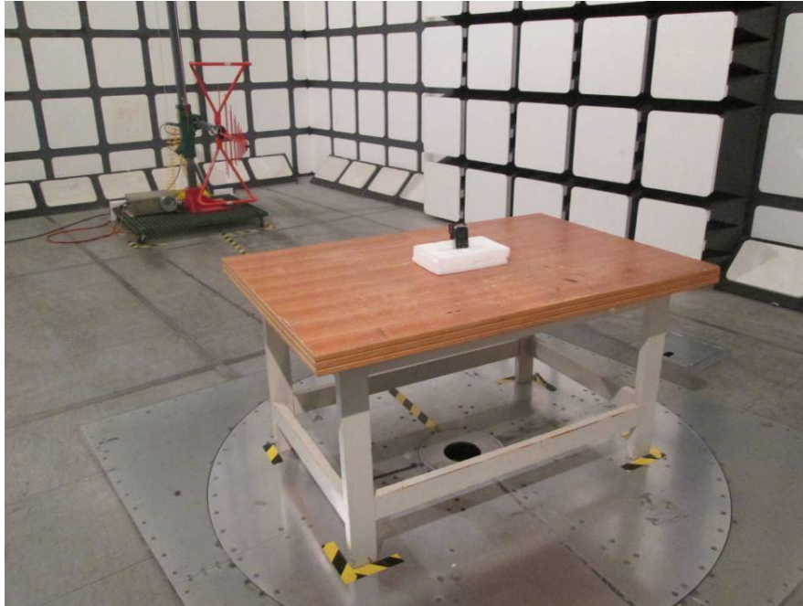
Radiated Emissions View (Below 1 GHz)
