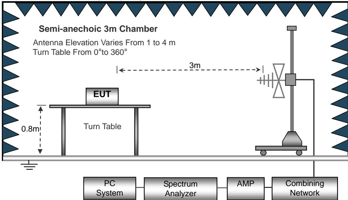
(C) Radiated Emission Test-Up Frequency Above 1GHz
