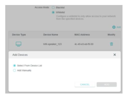
2. Select from the Device List or add devices manually in the Add Devices table. Enter the Device Name and MAC Address if you add devices manually.
