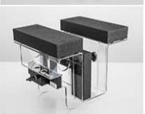
The DASY device holder is designed to cope with the different positions given in the standard. It has two scales for device rotation (with respect to the body axis) and device inclination (with respect to the line between the ear reference points). The rotation center for both scales is the ear reference point (ERP). Thus the device needs no repositioning when changing the angles.
