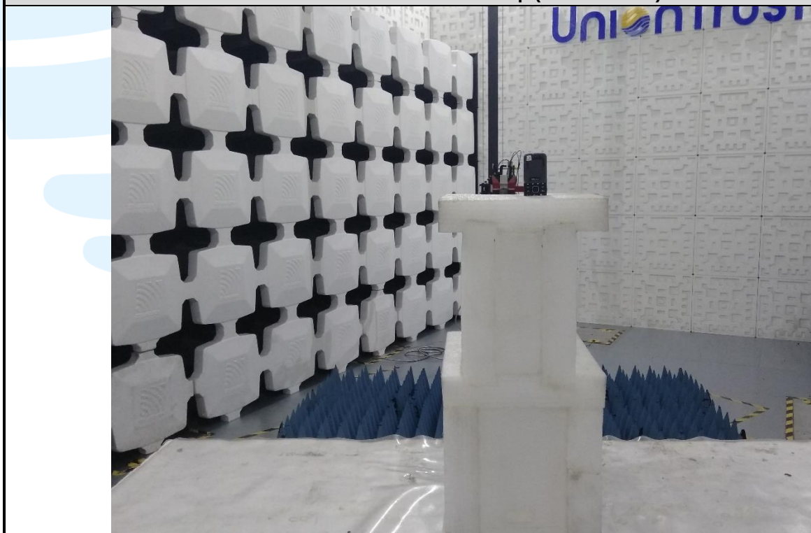
Radiated emission Test Setup (Above 1 GHz)
