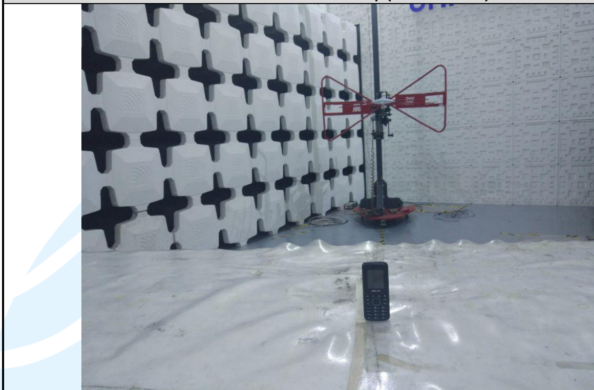
Radiated emission Test Setup (30 MHz~1 GHz)
