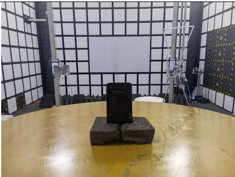
Spurious Radiated Emissions Test setup
