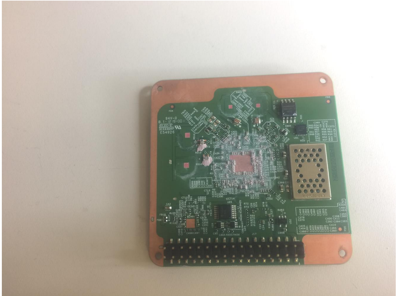
Figure 4 - Internal Photo of EUT- Main PCB with Shield Bottom View
