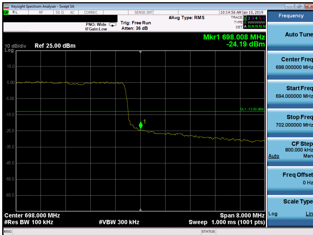
Plot 7-151. Upper Band Edge Plot (Band 71 - 10.0MHz QPSK - Full RB Configuration)
