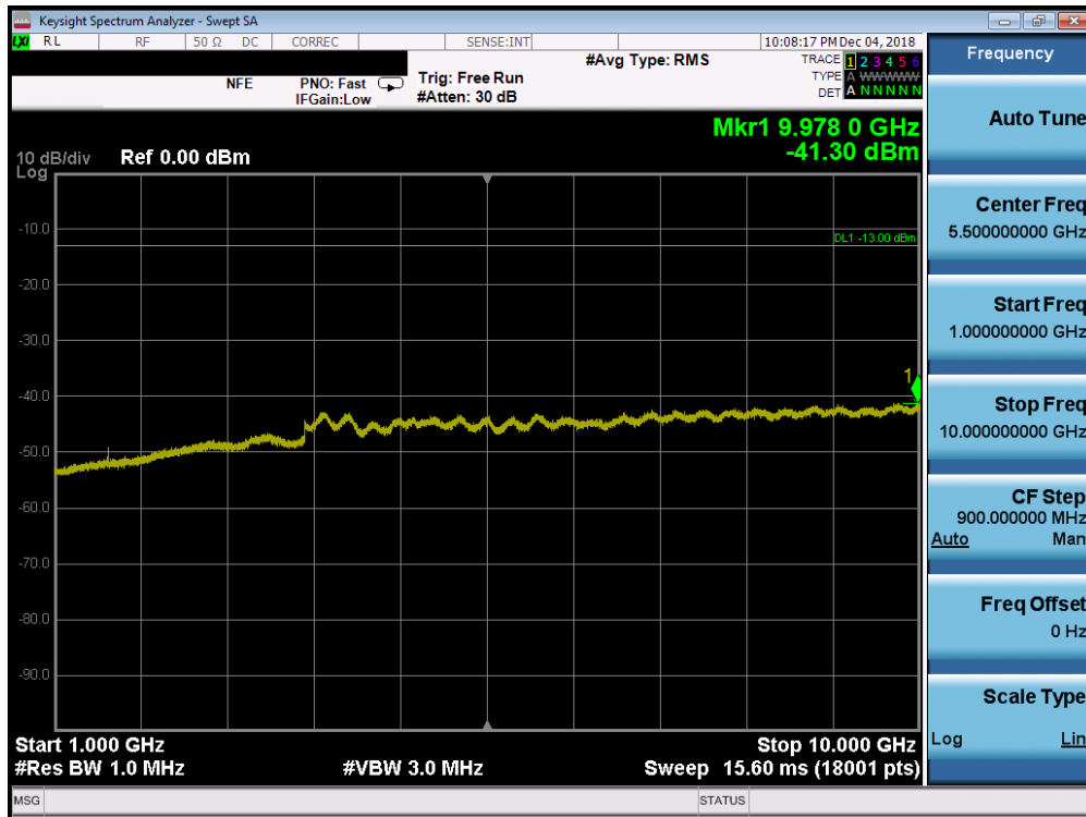
Plot 7-111. Conducted Spurious Plot (Band 13 - 10.0MHz QPSK - RB Size 1, RB Offset 0)
