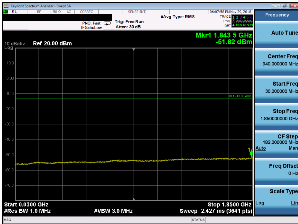
Plot 7-133. Conducted Spurious Plot (Band 25/2 - 10.0MHz QPSK - RB Size 1, RB Offset 0 - Mid Channel)
