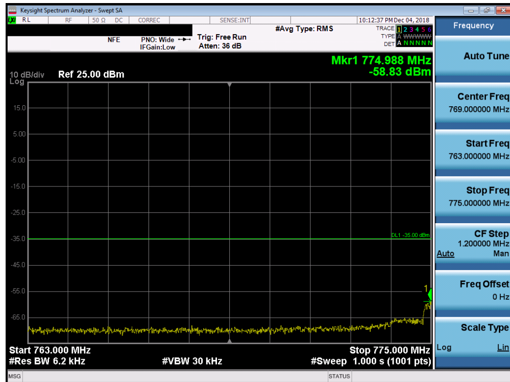
Plot 7-167. Lower Emission Mask Plot (Band 13 - 5.0MHz QPSK - Full RB Configuration)
