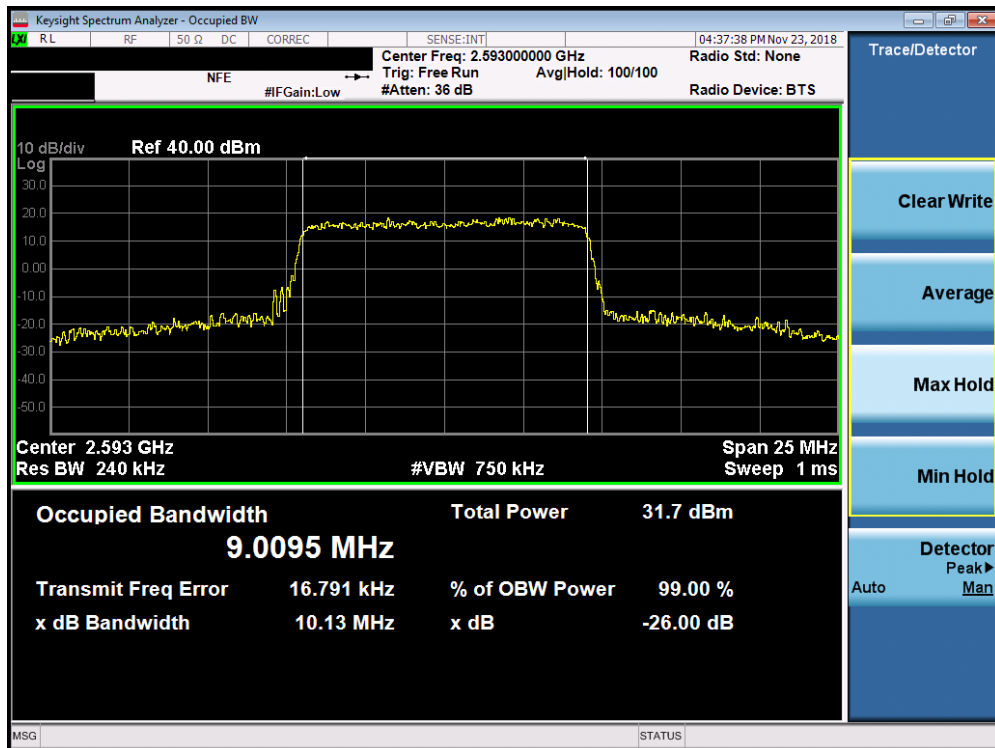
Plot 7-87. Occupied Bandwidth Plot (Band 41 (PC2) - 10.0MHz 64-QAM - Full RB Configuration)
