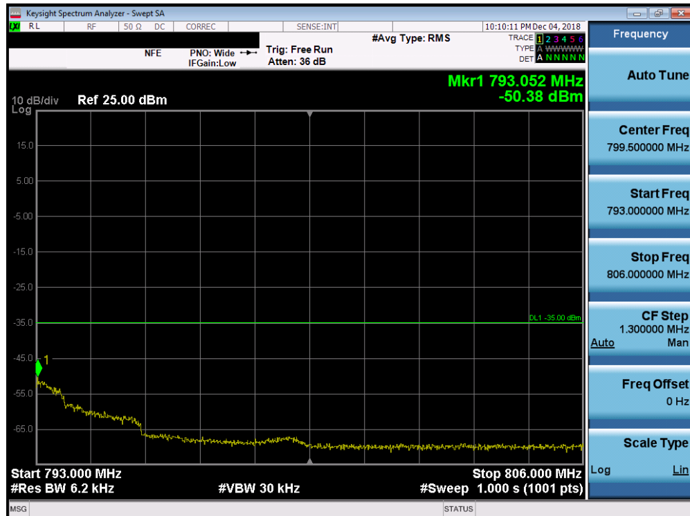
Plot 7-173. Upper Emission Mask Plot (Band 13 - 10.0MHz QPSK - Full RB Configuration)
