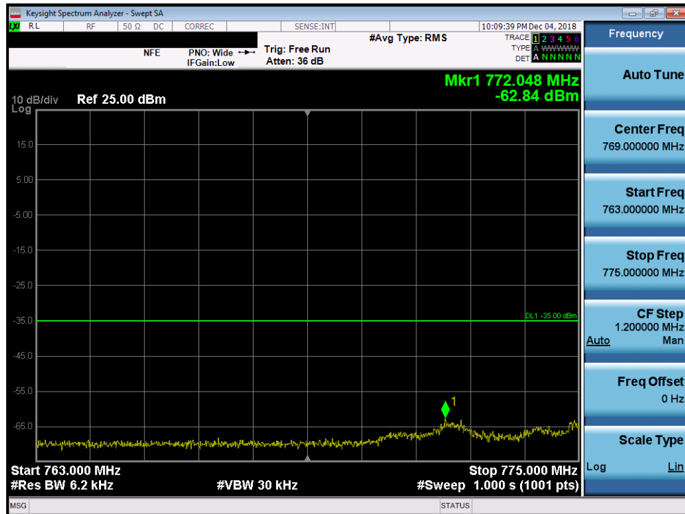
Plot 7-171. Lower Emission Mask Plot (Band 13 - 10.0MHz QPSK - Full RB Configuration)
