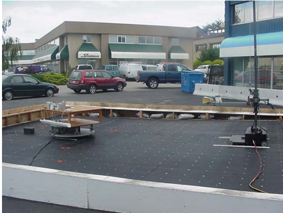
Photograph F-1 - 3115 Horn with LNA/filter @ 3 m
