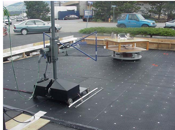
Photograph G-4 - 3115 Horn with LNA/Filter @ 1m
