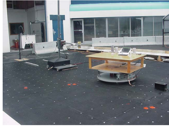
Photograph F-2 - 3115 Horn with LNA/Filter @ 1m
