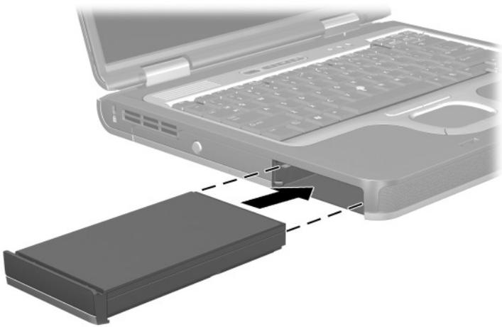
To remove a battery pack, turn the notebook upside down. Slide and hold the battery release latch **1** as you pull the battery pack **2** from the battery bay.
