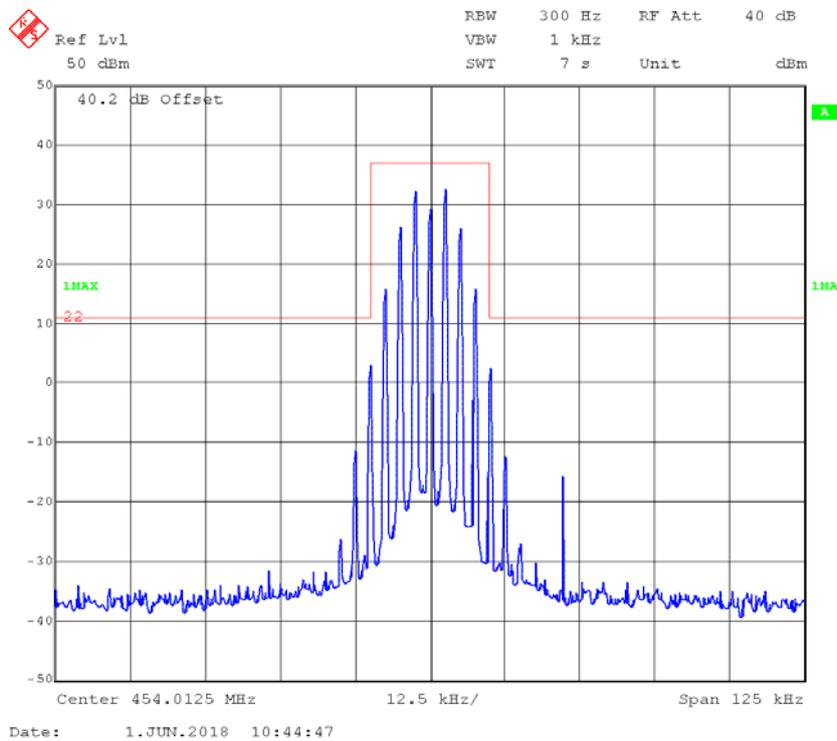
**4FSK,12.5kHz,High Power - Frequency 454.0125 MHz: 99% Occupied & 26 dB Bandwidth**
