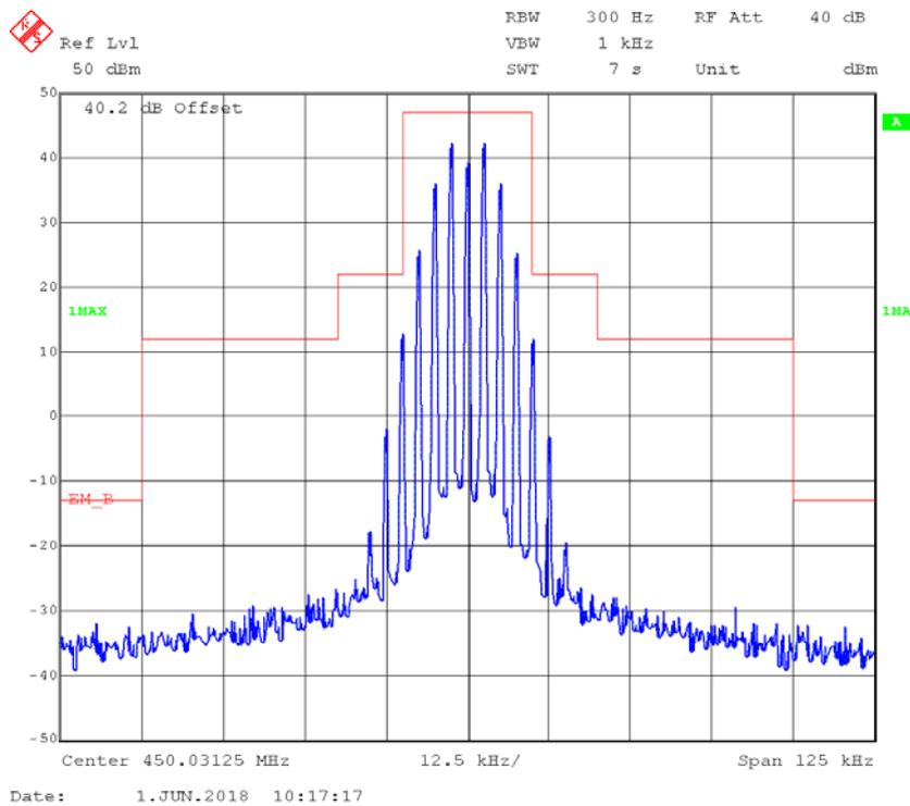
**4FSK,12.5kHz,Low Power - Frequency 450.03125 MHz: 99% Occupied & 26 dB Bandwidth**
