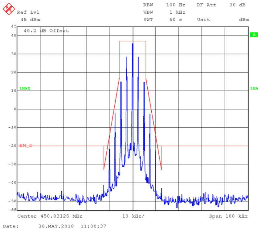
**FM,25kHz,High Power - Frequency 450.03125 MHz: 99% Occupied & 26 dB Bandwidth**
