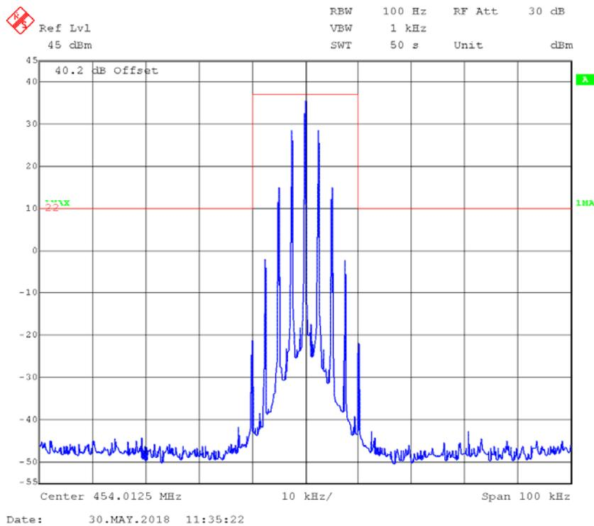
**FM,25kHz,High Power - Frequency 454.0125 MHz: 99% Occupied & 26 dB Bandwidth**
