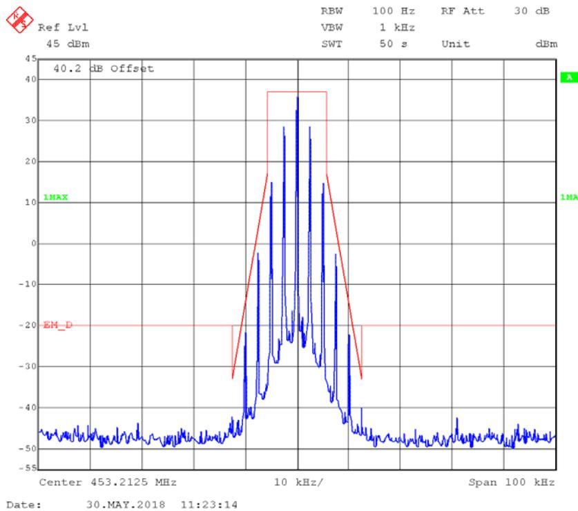
**4FSK,12.5kHz,High Power - Frequency 453.2125 MHz: 99% Occupied & 26 dB Bandwidth**
