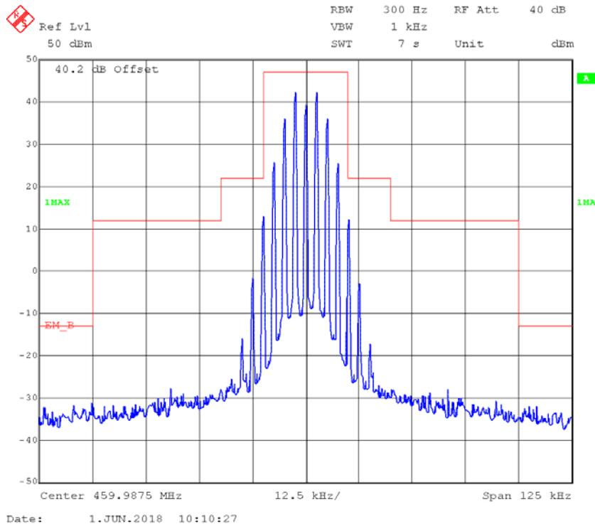
**FM,25kHz,Low Power - Frequency 459.9875 MHz MHz: 99% Occupied & 26 dB Bandwidth**
