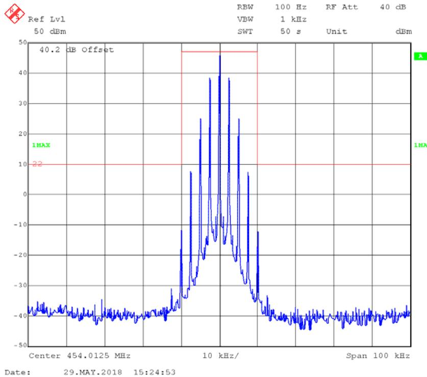
**FM,12.5kHz,Low Power - Frequency 454.0125 MHz: 99% Occupied & 26 dB Bandwidth**
