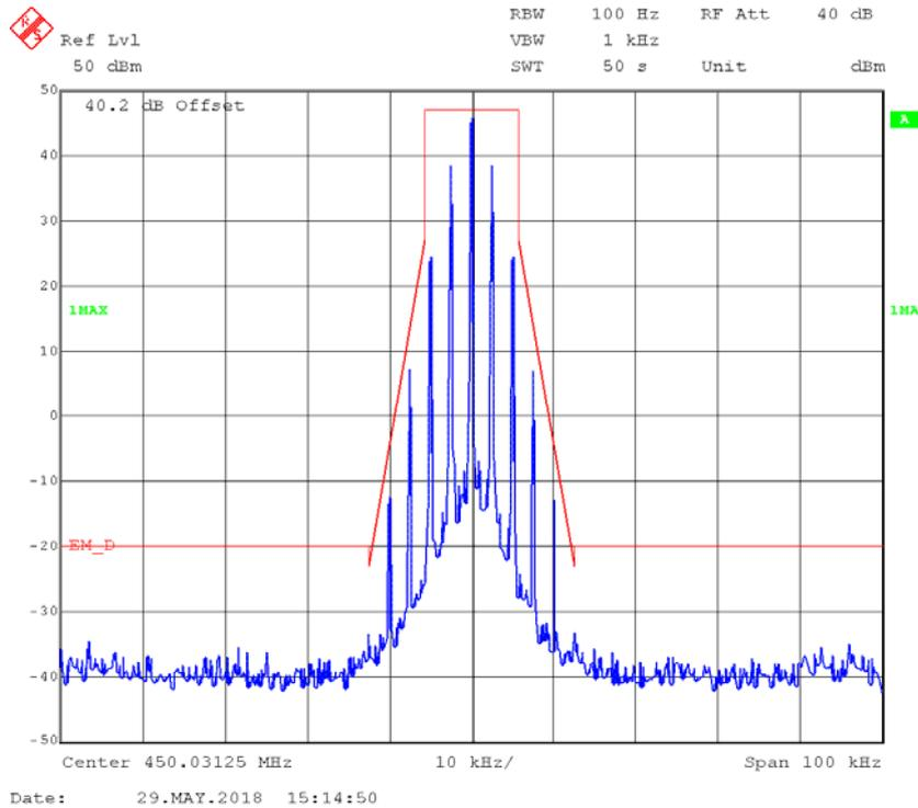
**FM,12.5kHz,Low Power - Frequency 450.03125 MHz: 99% Occupied & 26 dB Bandwidth**
