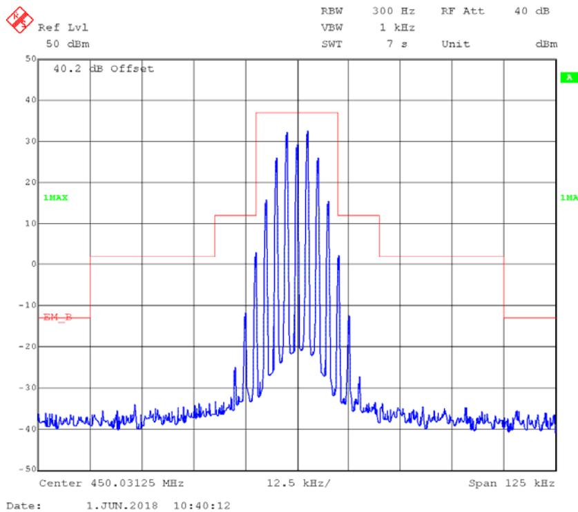
**4FSK,12.5kHz,High Power - Frequency 450.03125 MHz: 99% Occupied & 26 dB Bandwidth**
