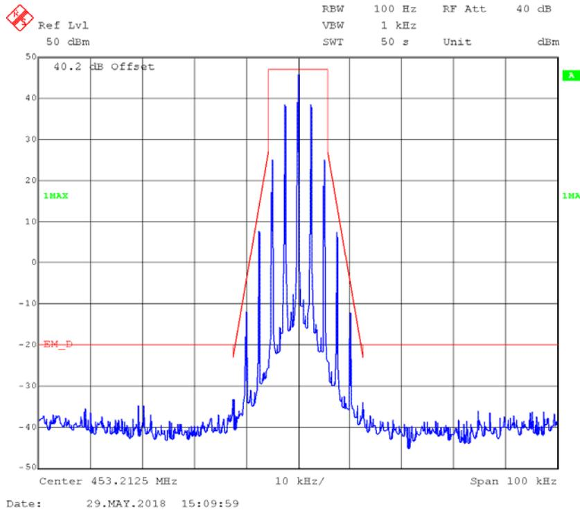
**FM,12.5kHz,Low Power - Frequency 453.2125 MHz: 99% Occupied & 26 dB Bandwidth**
