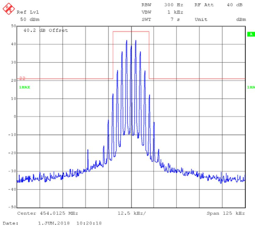
**FM,25kHz,Low Power - Frequency 454.0125 MHz: 99% Occupied & 26 dB Bandwidth**
