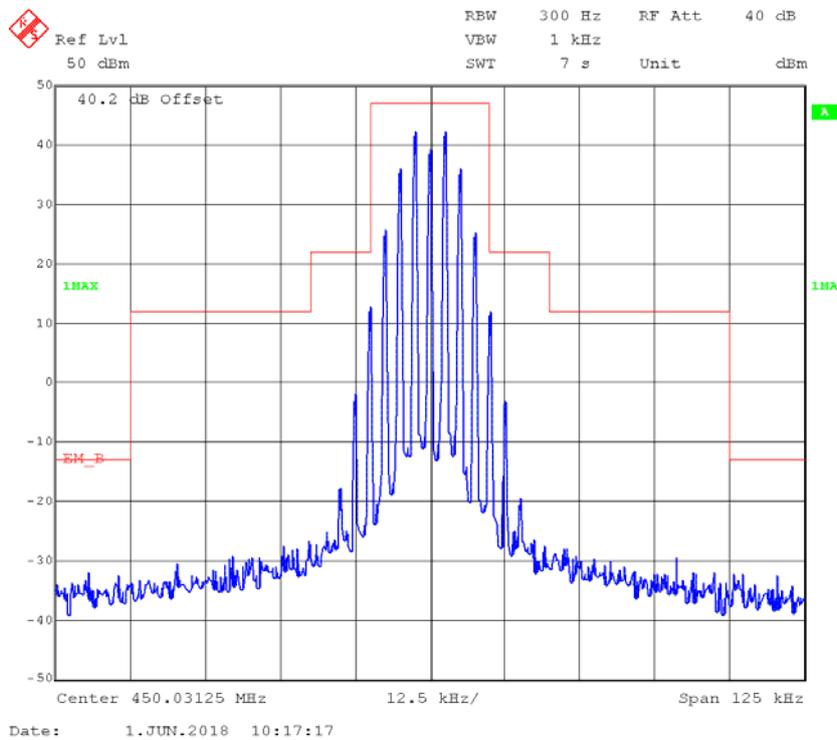
**FM,25kHz,Low Power - Frequency 450.03125 MHz: 99% Occupied & 26 dB Bandwidth**
