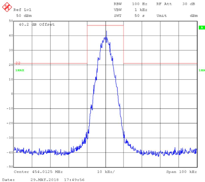
**4FSK,12.5kHz,Low Power - Frequency 454.0125 MHz: 99% Occupied & 26 dB Bandwidth**
