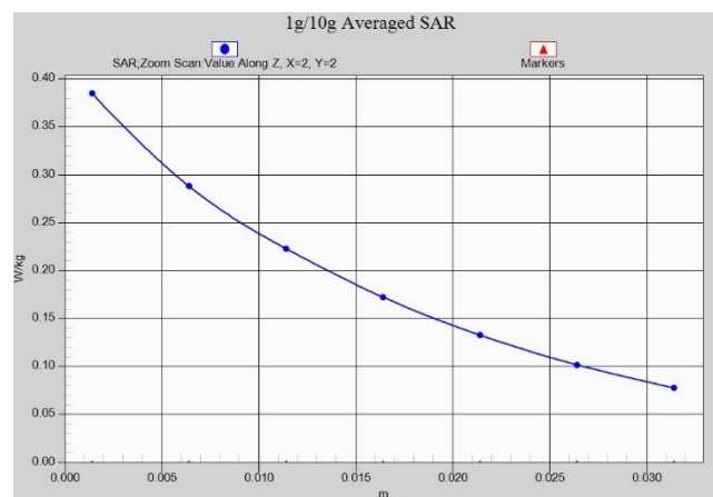
Fig. 1-26Z-Scan at power reference point (LTEB28)
