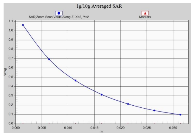
Fig. 1-13Z-Scan at power reference point (WCDMA850)
