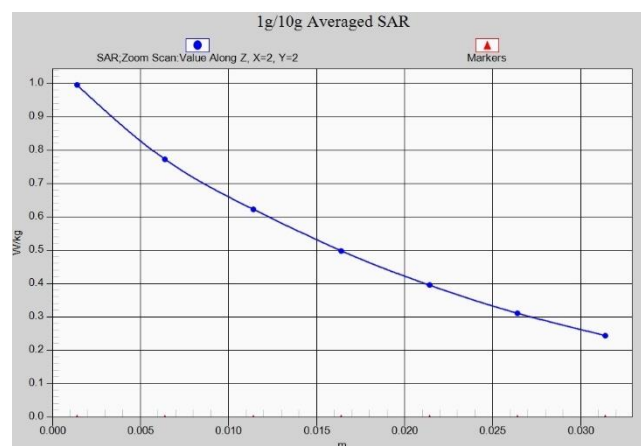
Fig. 1-12 Z-Scan at power reference point (WCDMA850)
