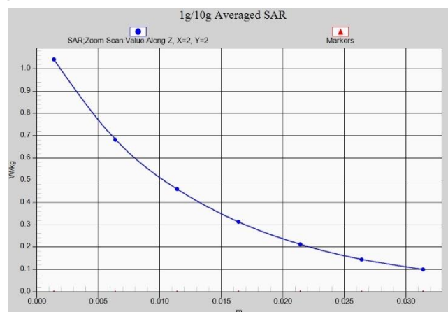
Fig. 1-6 Z-Scan at power reference point (WCDMA1900)
