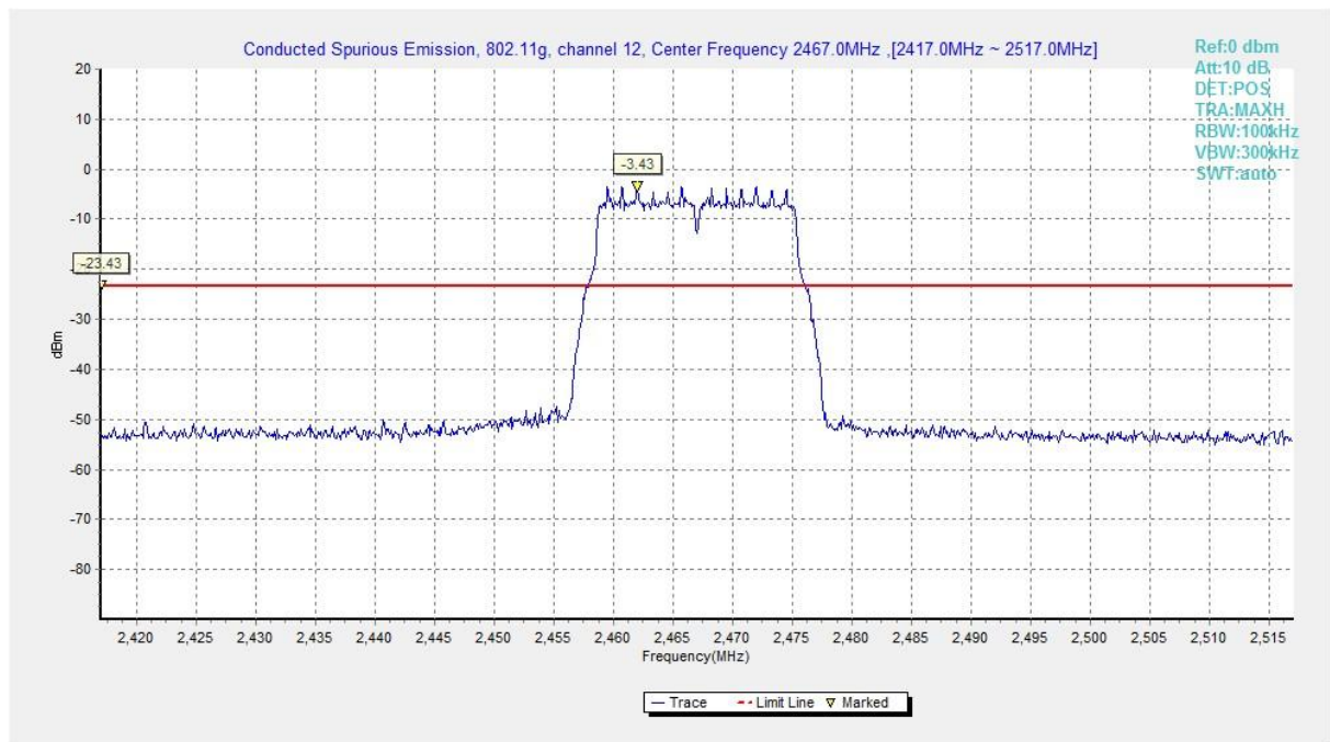
Fig.A.6.1.65 Conducted Spurious Emission (802.11g, Ch12, Center Frequency)
