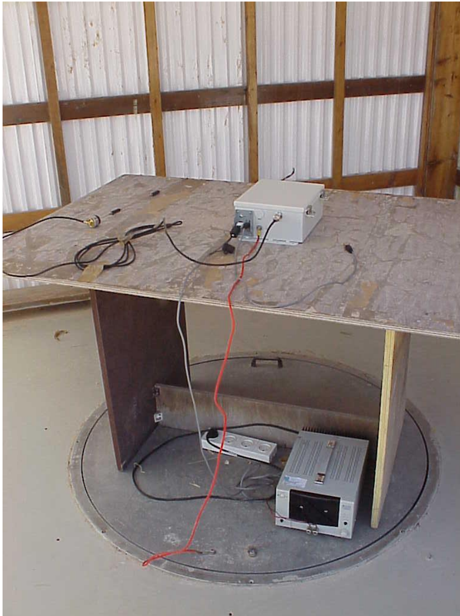
Photo 2. BreezeAccess SU-M-900 Radiated emission test setup at open site
