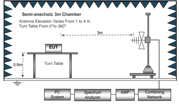
(C) Radiated Emission Test-Up Frequency Above 1GHz
