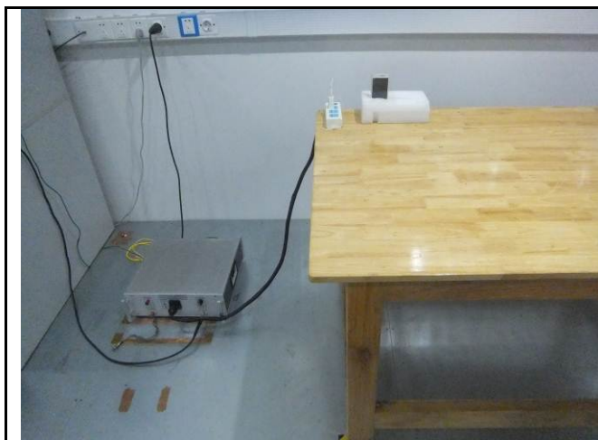
Conducted Emissions Test Setup Front View
