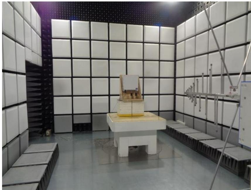
1.2 Radiated emissions set-up for frequencies above 1 GHz
