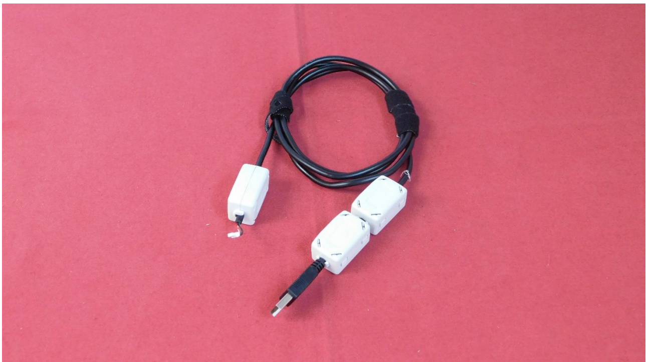
Picture 12: USB cable with ferrites
