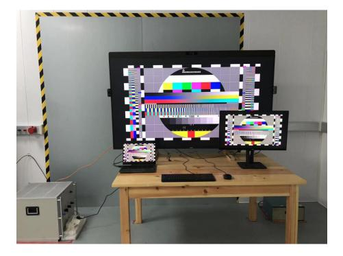
Radiated Emission Test Setup Photo - Below 1GHz
