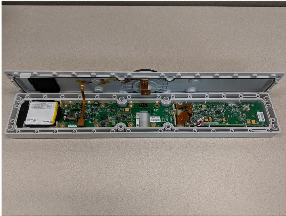
EUT Battery + PCB View
