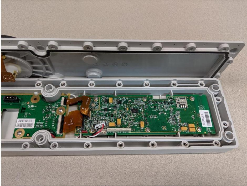
Shield Part Removed for C2PC
