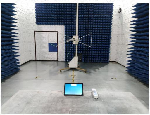
FCC RADIATED EMISSION TEST SETUP ABOVE 1GHZ
