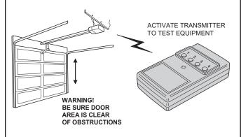
Description The Delta-3 DT-4B digital transmitter is a four-channel wireless radio control designed for use with automatic garage/gate operators and access control systems. The transmitter can be used with one 4-channel receiver (DR4), two 2-channel receivers (DR2) or four single-channel receivers (DR,DRQ or DRM). Receivers should be mounted at least 8 feet apart.
