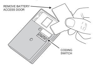
STEP 2C: Coding for a four-channel receiver. Pick any combination of OFF/ON codes, and set them on switch keys 3-8 in the transmitter. Match the same code on switch keys 3-8 in each receiver. Transmitter and receiver switch keys 1 & 2 are unused and can be in any position.
