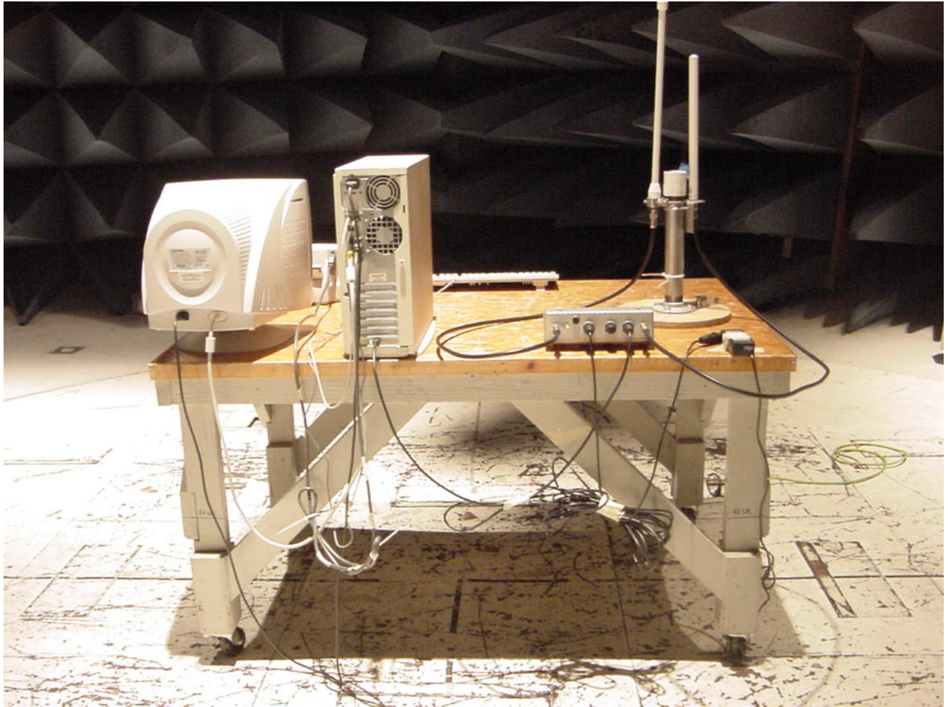
Photograph 2. Radiated Emission Test Setup < 1 GHz
