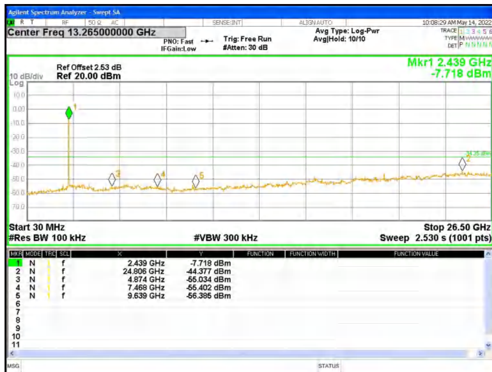
Tx. Spurious NVNT n20 2462MHz Ant1 Ref
