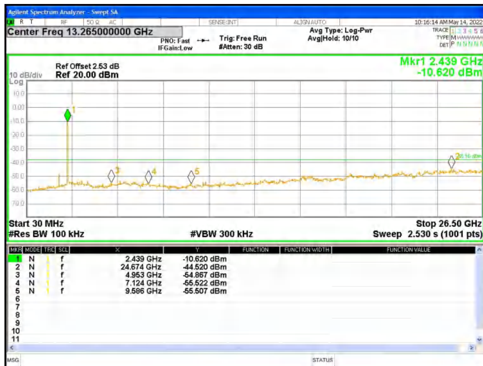
Tx. Spurious NVNT n40 2452MHz Ant1 Ref
