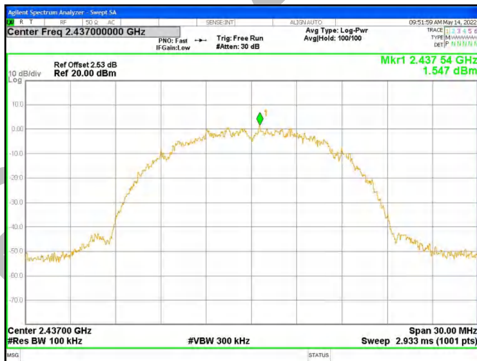
Tx. Spurious NVNT b 2437MHz Ant1 Emission
