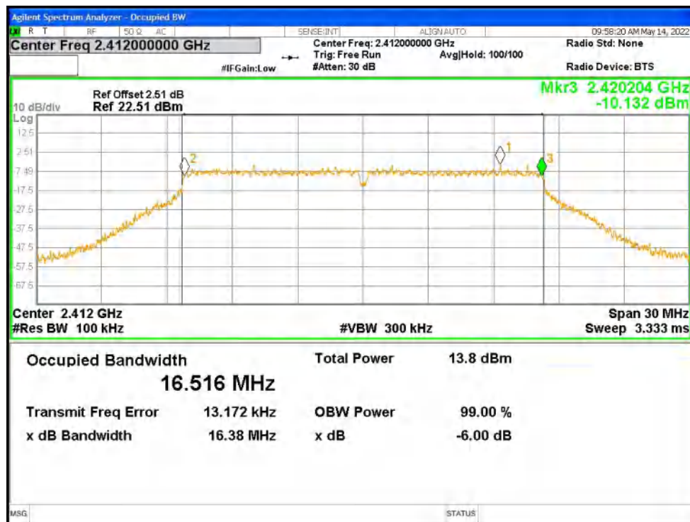
-6dB Bandwidth NVNT g 2437MHz Ant1
