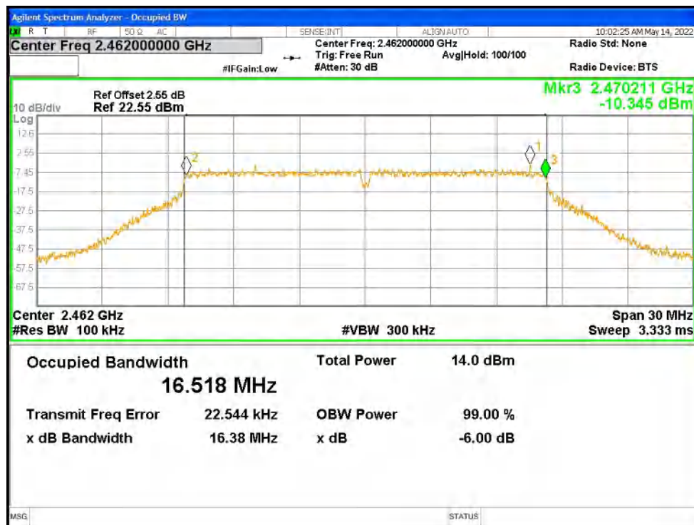
-6dB Bandwidth NVNT n20 2412MHz Ant1
