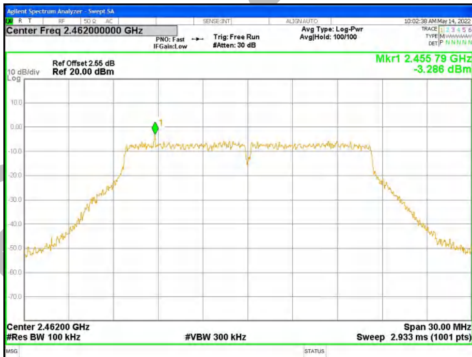
Band Edge NVNT g 2462MHz Ant1 Emission
