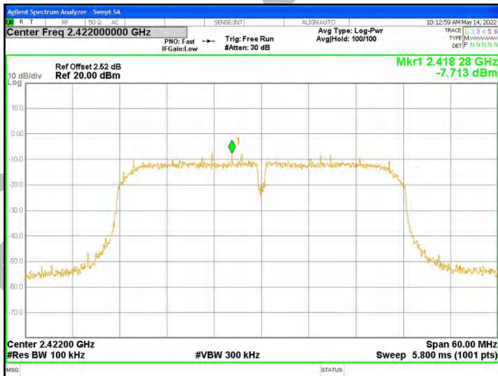
Band Edge NVNT n40 2422MHz Ant1 Emission
