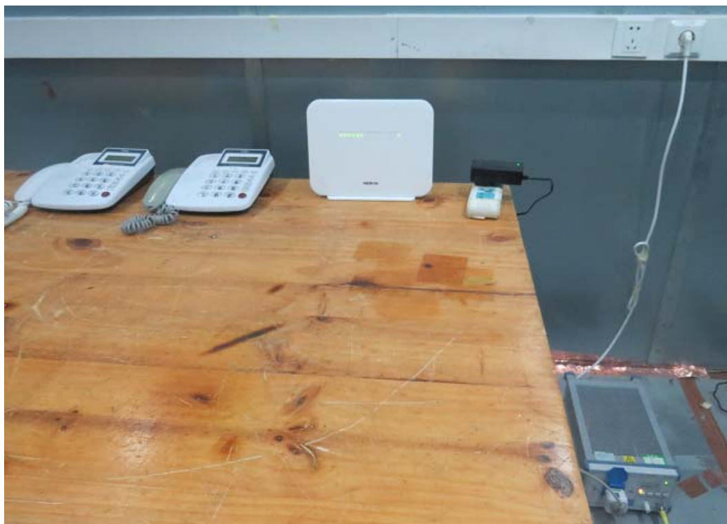
Picture 2 Conducted Emission Test Setup
