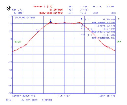
Plot # 4: 99% OBW, RF Output Frequency: 901 MHz, Modulation: 2-Level 8kbps GMSK
