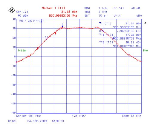
Plot # 5: Emission Mask J, , RF Output, High Power Setting Frequency: 896 MHz, Modulation: 2-Level 8kbps GMSK
