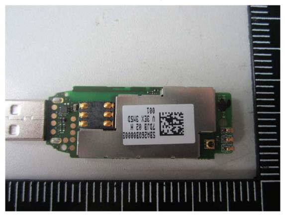
3. Mainboard rear view with shielding
