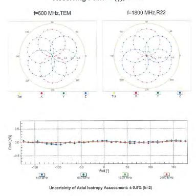
Receiving Pattern ( $\phi$ ),  $\vartheta = 0^{\circ}$
