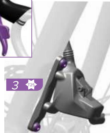
Loosely install the caliper onto the fork. Lightly squeeze (approx. 4 lbs.) the lever blade repeatedly to advance the caliper pistons, then hold the lever blade and lightly tighten the bolts.
