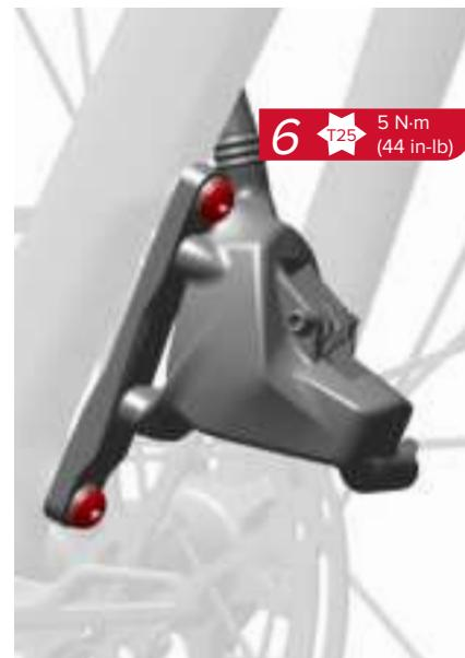
Check that the brake pads are equally spaced on either side of the rotor, lightly squeeze (approx. 4 lbs) and hold the brake lever, and then tighten the bolts to the torque specified.
