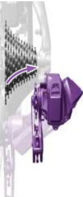
Press the right shifter paddle to move the rear derailleur outboard to a smaller cog. Press and hold the paddle for multiple shifts.
