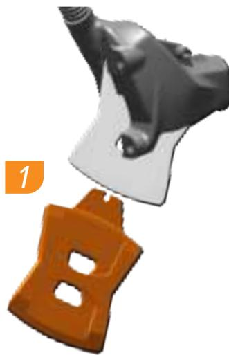
Remove the pad spacer from the caliper.
