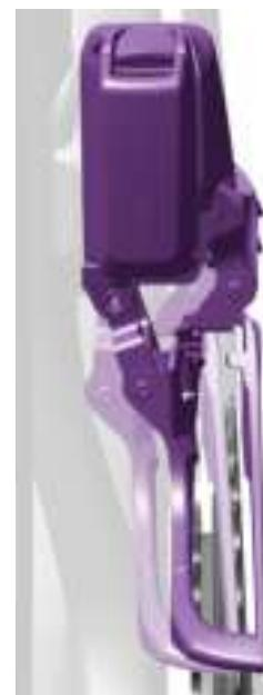
**For 2x systems:** press both shifter paddles simultaneously to move the front derailleur inboard or outboard.
