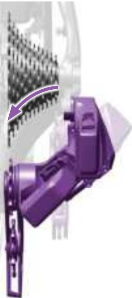
Press the left shifter paddle to move the rear derailleur inboard to a larger cog. Press and hold the paddle for multiple shifts.
