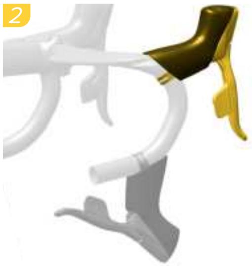
Install the shift-brake lever onto the handlebar and set it to your desired position.
