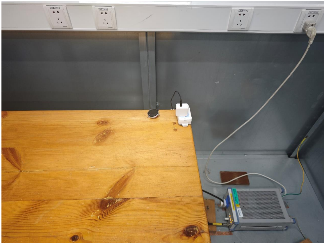
5. Conducted Emission (Part 15B, Bluetooth/Video Player)
