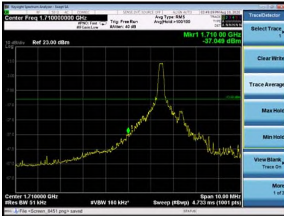
LTE Band 4 16QAM 20MHz CH-Low, 100%RB
