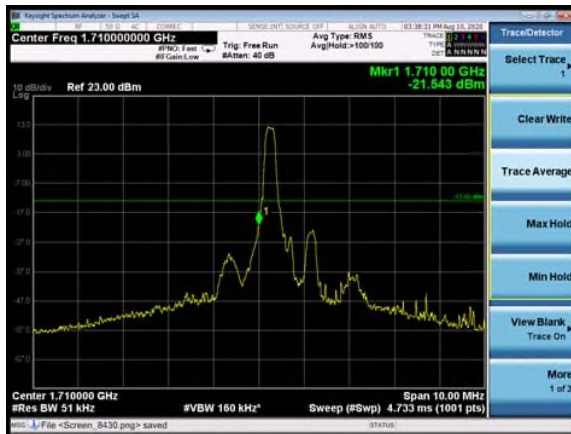
LTE Band 4 16QAM 1.4MHz CH-Low, 100%RB
