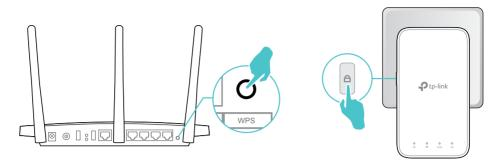
2. Wait until the Signal LED changes to solid on, which indicates that the WPS connection is successful.
