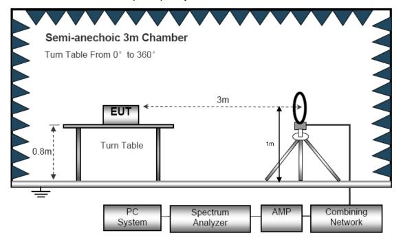
(B) Radiated Emission Test-Up Frequency 30MHz~1GHz
